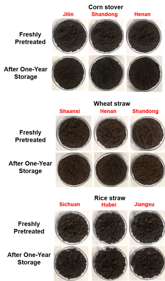
Figure 2. Morphological observation of the freshly pretreated and year-round stored crop residue feedstocks in different regions.
